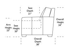
\*Note: arm height for this frame is measured at the highest point of the curved arm.
